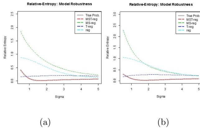
Figure 5: The distance between true model and alternative model under perturbations in sigma parameter
