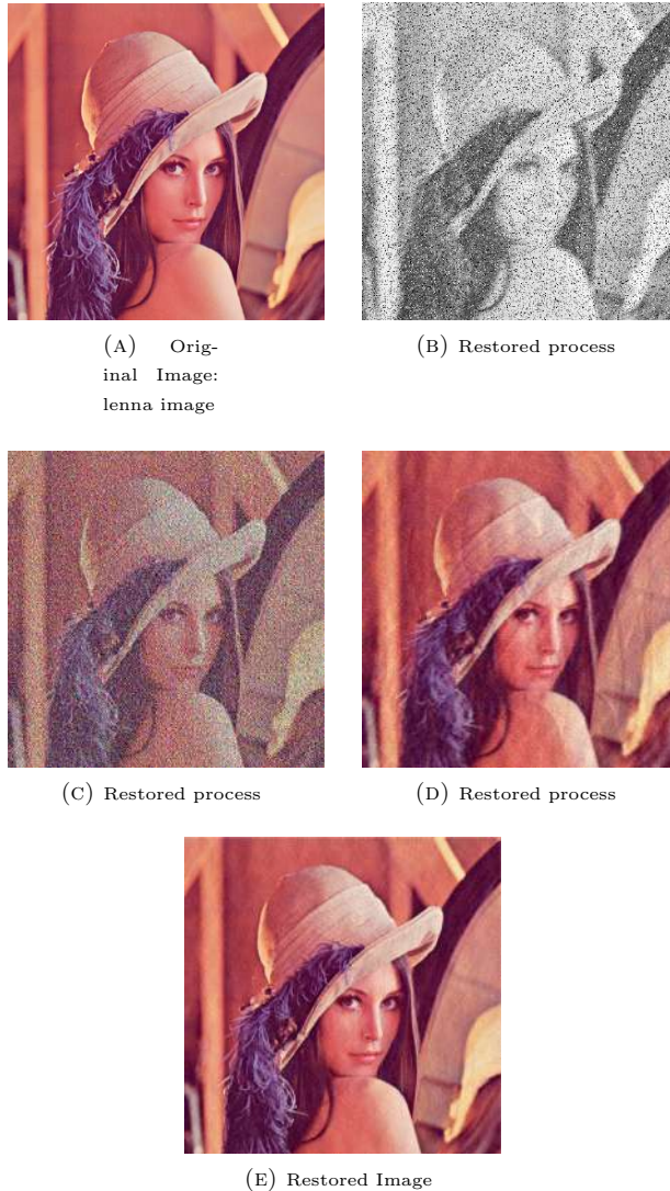
FIGURE 21. The image degradation and restoration using Wiener filter
